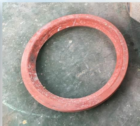
Corroded Rubber Seal Ring
