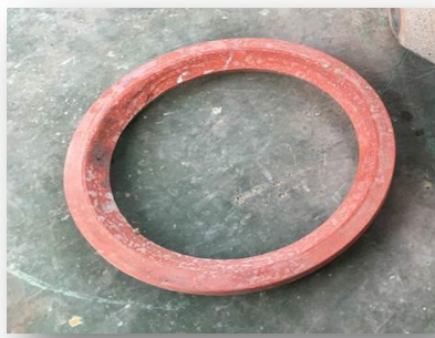
Corroded Rubber Seal Ring
