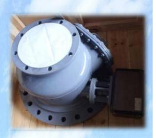
swing cylinder. The cylinder drives damper arm through rotary shaft and damper arm connect with damper plate.
